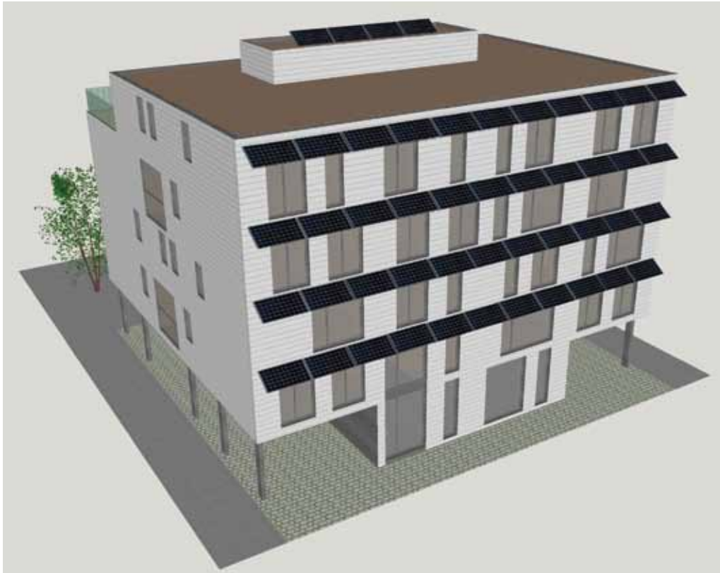
Figure 3.15. PV panels as shades on the south façade
